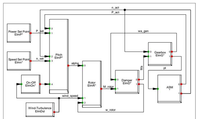
Figure 4: Wind turbine controller model
