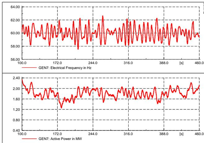
Figure 7: Base case simulation – Frequency and generator power
