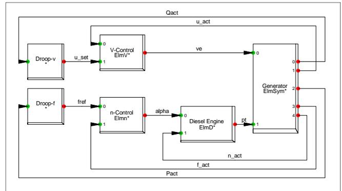
Figure 3: Generic generator controller model
