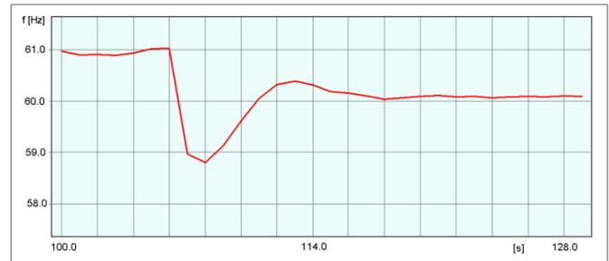
Figure 9: 2MW step response of the real system
