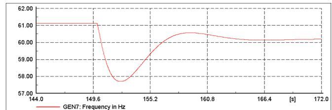
Figure 10: 2MW step response of simulation model
