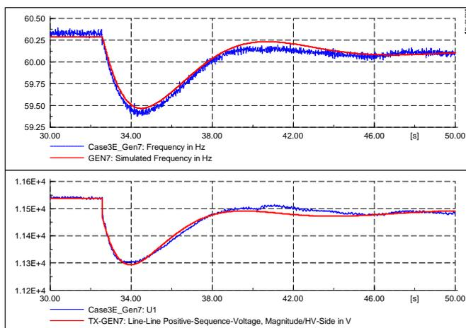
Figure 5: Generator step response (blue-real; red-simulation)
