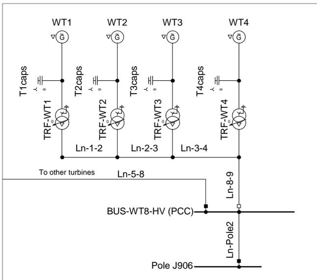
Figure 2: Windfarm model in PowerFactory
