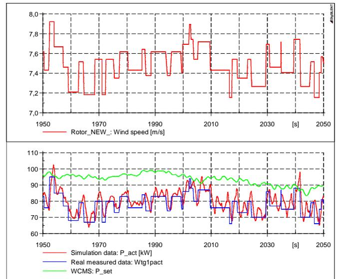
Figure 6: Wind turbine response (blue-real, red-simulation, green-set point)
